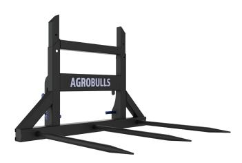
Used for Carrying and Stacking Prismatic Large Hay and Straw Bales. The large bale fork is designed for loading and carrying hay, haylage or similar materials. The load should be taken with two teeth at the same time.
