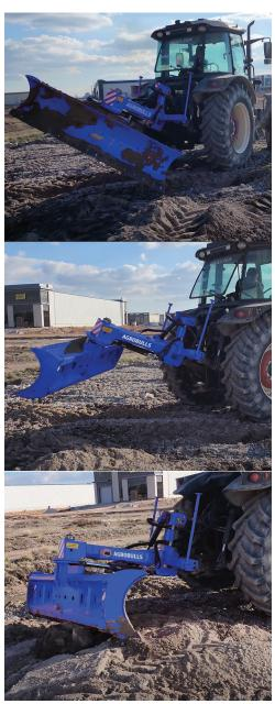
It is used in agriculture, forestry and construction sectors, suitable for repairing roads, water channels and agricultural land borders. It is also used to clear snow on forest roads and in places that are difficult to reach for snowplows.
