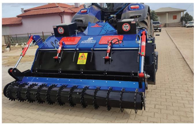
Our machine; The tractor takes motion from the PTO. It is connected to the tractor hydraulic suspension arms. On the field surface and 20-60 cm underground breaks stones with diamond blades.
